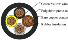
Polychloroprene rubber outer jacket Bare copper conductor
